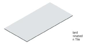
Abtech Cleanroom Ceiling Tiles are used to seal spaces in the T-Grid System not occupied by a Lighting Fixture or Fan Powered Filter Unit. Nominal Sizes are 24" x 48" x 1/2" (23 3/4" x 47 3/4" actual). Material choices include Vinyl Laminated Gypsum, Aluminum, and Fiberglass Reinforced Plastic (see opposite for detailed descriptions).
